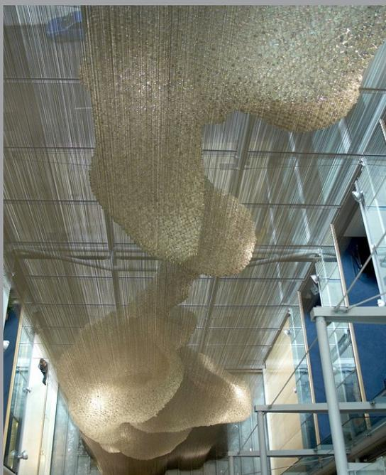
Almost a million metres of high tensile strength wire were used for suspension and Ormiston was commissioned to provide a solution with the strength to support a staggering 15 tonnes of glass above a pool of water that would also provide the required aesthetic appeal.
