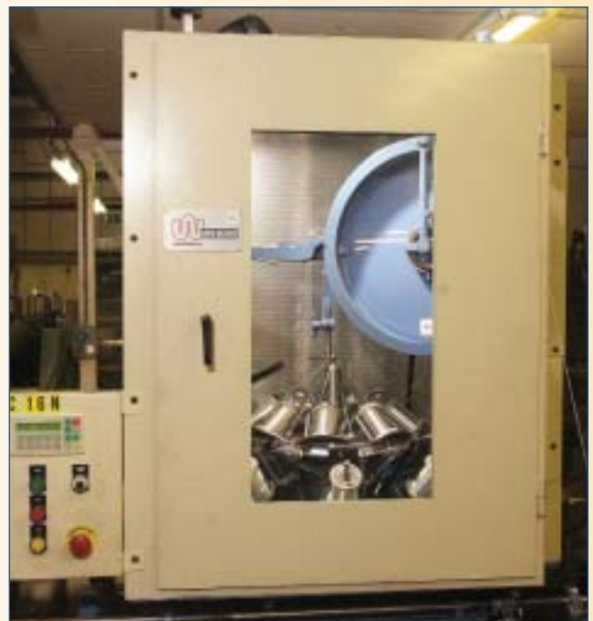
Efficient: The braider works through the night without the need for an operator
